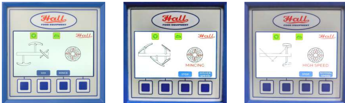
NG i-DAS with VSD Installed - Normal Speed / High Speed
